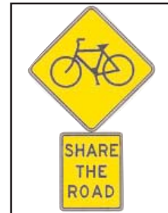
figure 3.9 W11-1 sign with "Share the Road" plaque to be installed prior to right turn lanes
